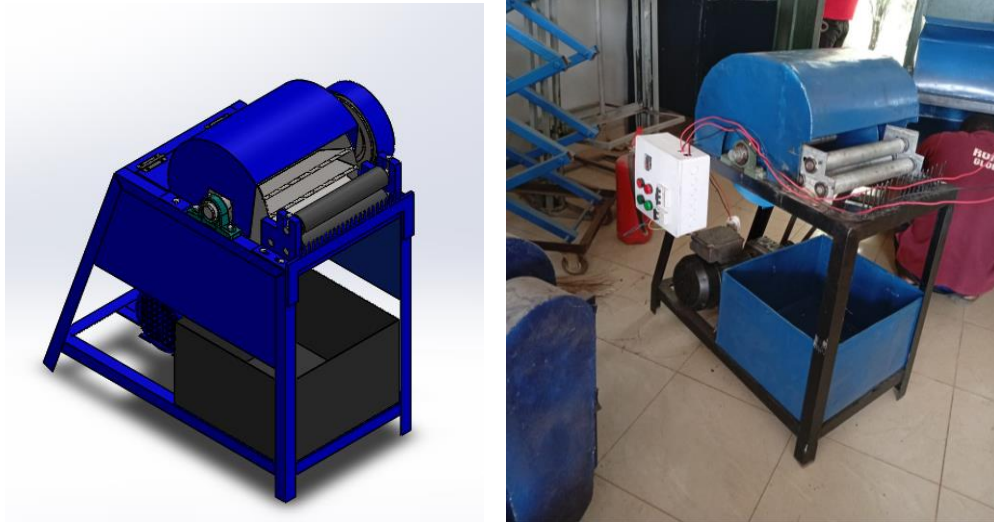
Fig. 1: Pictorial view of the locally produced plantain/ banana fiber extraction machine.
