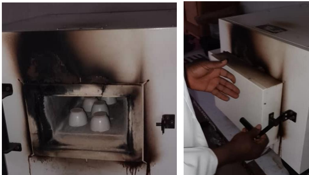
Figure 4 [a], [b]: Sintering of the membrane at the muffle furnace.
