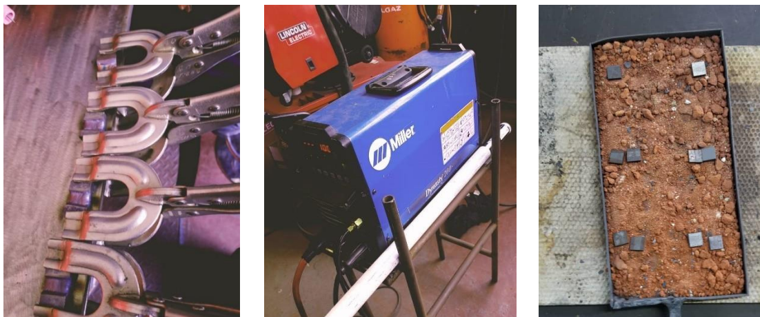
Figure 2: Clamps used to grip the sample, TIG Welding Machine, and Samples in Rectangular furnace Tray
